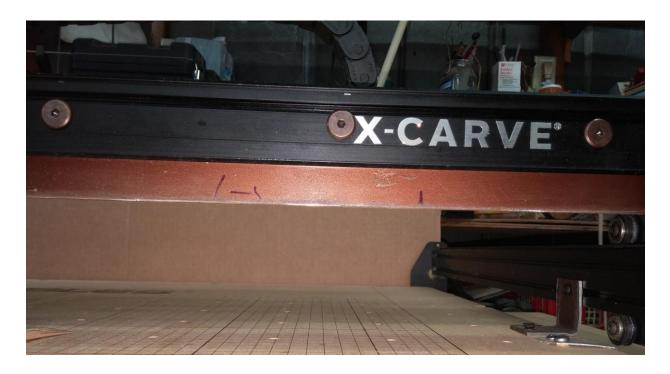
Before you start, power your machine up and check to see just how much flexing or twisting the Maker slides have by pulling forward on the bottom of the spindle and pushing backward on the top at the same time. Don't go all gorilla here, don't want to break anything! You will find that the bottom of the spindle moves far more than would be desired. (Powering it up will help to hold things still while you check this). Repeat this at the end of the upgrade and be amazed at the difference!
