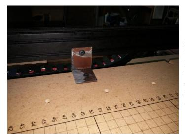
One other area that needs attention is the long Y rails. To insure that these don't bow under load I installed one L bracket at the mid point of each rail. I used some angle iron to insure that I had a good solid anchor for them. A word of caution. Be sure to position the brackets firmly against the rails. You as don't want to cause the rails to bow in / out / or downward when tightening them.
