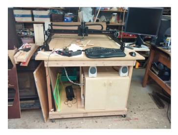
When running the machine I keep the doors closed to keep the dust and debris out of the sensitive electronics. This includes an air filter and both a sucustion and blowing fans to circulate the air inside the cabinet.
