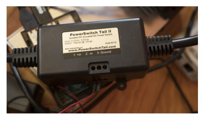
Plug the power cord from the X-Carve power supply into the Powerswitch Tail, and then plug in the Powerswitch Tail into an outlet. Flip the X-Carve power supply into the on position, and plug in your Raspberry Pi to a power outlet. From now on the Raspberry Pi will be controlling the power to your X-Carve.
