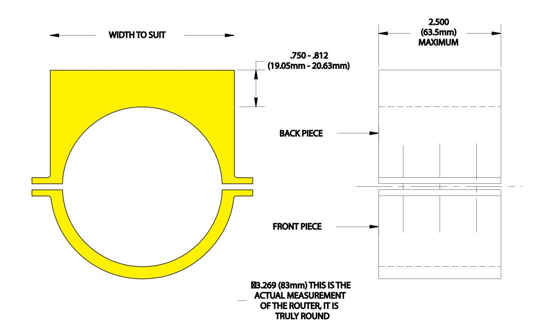
I WOULD LIKE TO HAVE A TWO PIECE DESIGN SO THAT I CAN DRILL THE MOUNTING HOLES FROM THE BACK OF THE BACK PIECE AND COUNTERBORE FOR TEE NUTS OR THREADED INSERTS FROM THE FRONT OF THE BACK PIECE.
