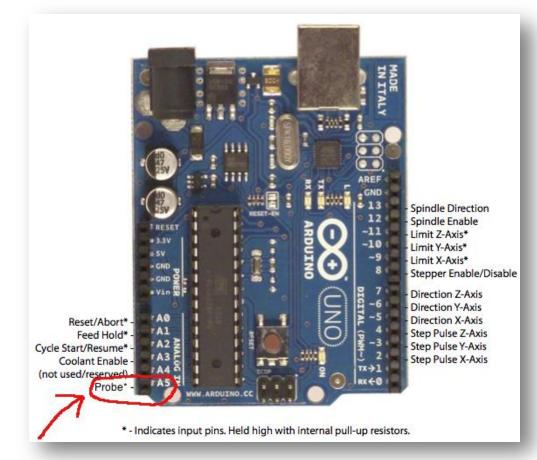
4. Route this wire to a location of your choice. Some like to use a plug of sorts so they can remove their touch plate wiring when not in use. This wire will eventually be connected to the touch plate.
